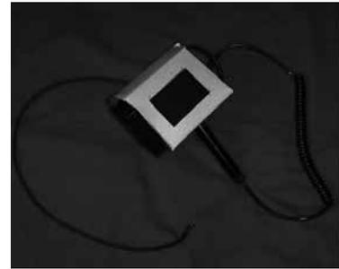
**Figure 1.** Borescope with pistol-style grip. Borescopes of this style are widely available from a number of manufacturers
